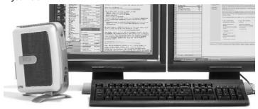
The mid-range Wyse V90L thin computer delivers the Windows XPe performance you need; dual-video support (with purchase of optional monitor splitter cable); a CardBus/PCMCIA slot; plus serial, parallel, and USB ports. Options include internal WiFi solution and smart card slot. Using the same form-factor as the Wyse V90, the Wyse V90L can fit easily into most work environments.
