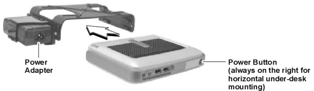
6. Attach the power adapter holder to the wall bracket using the two (2) M3x8 mm screws provided and slide or rotate the thin client's power adapter into the power adapter holder.
