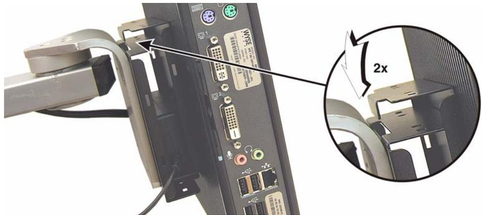
6. Line up the screws holes of the bracket pieces (two on top and two on bottom) and secured with four (4) four thumb screws provided (do not overtighten).
