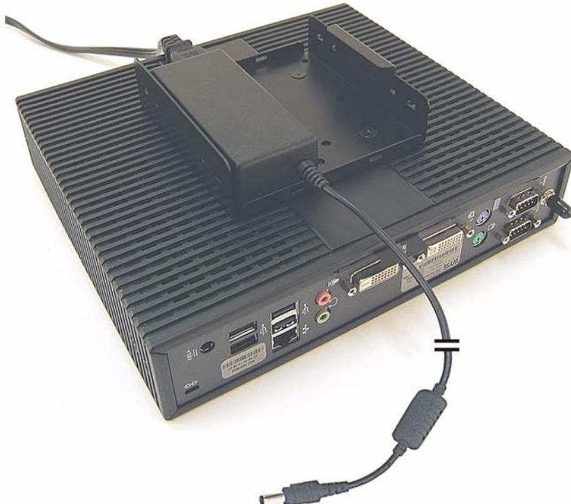
4. Attach the second bracket piece to the mounting surface (a swing arm mount is shown). The mounting surface can have either the VESA 75 mm or 100 mm mounting pattern. If the mounting surface is a pole, stud, or beam, use the center vertical or horizontal mounting holes. The bracket should be placed with the slotted end on top and with the turned edge at the bottom (pointed upward). Secure the bracket with proper user-provided hardware that can withstand a force of 35 pounds.
