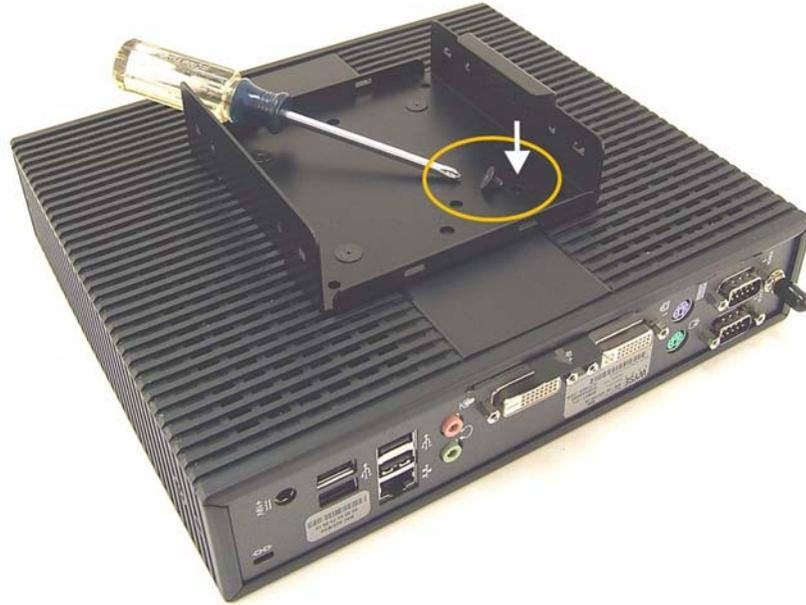
3. Place the power supply on the bracket that is attached to the thin client, with the AC power cord facing toward the front of the thin client and DC cord facing the back panel side.
