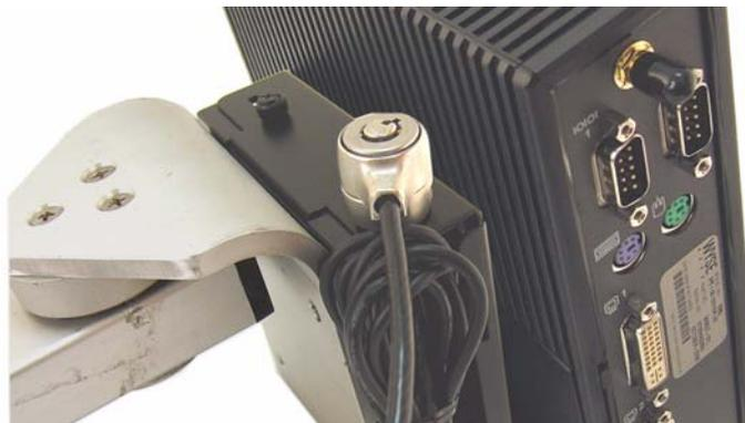
9. Attach the cables to their respective connectors on the back panel of the thin client.
