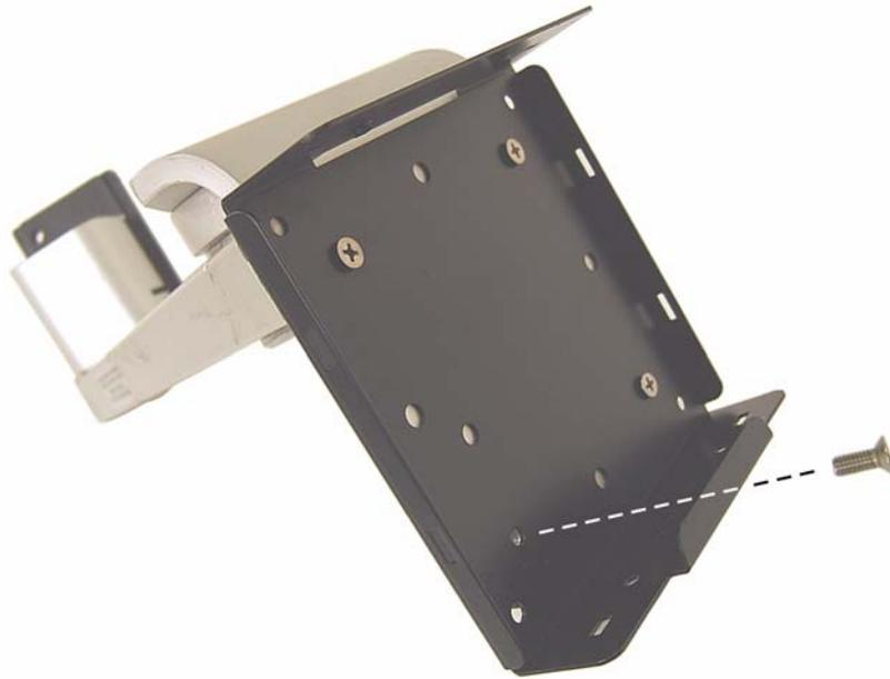
5. Face the thin client's bracket toward the mounted bracket. Hold the thin client a little higher than the mounted bracket, and then slide it downward to have the bracket's turned edges drop into slots at both top and bottom.
